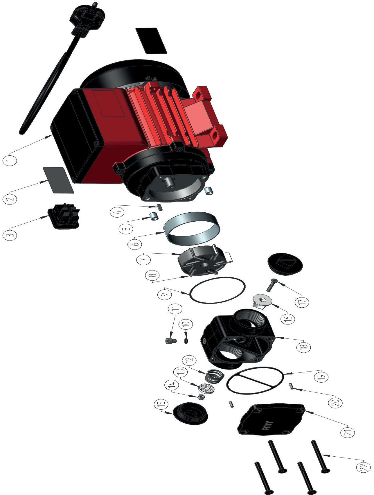
Fig. 15. - 1: Exploded view of the diesel pump 60 l/min
